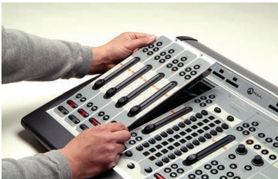
Figure C-15: Tilt module up to remove from frame.
