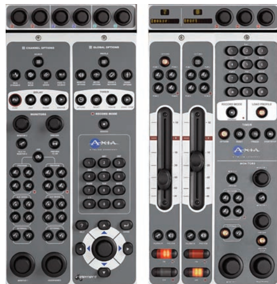
Figure 1-6: Identifying the Standard Monitor Module (left) and Monitor + 2-Fader Module (right).
