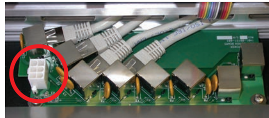
Figure 1-5: Element connection panel. Circled connector is for power/data cable; RJ-45’s connect to fader and accessory modules.
