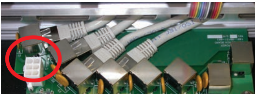
Figure 2-9: Element connection panel. Circled connector is for power/data cable; RJ-45's connect to fader and accessory modules.
