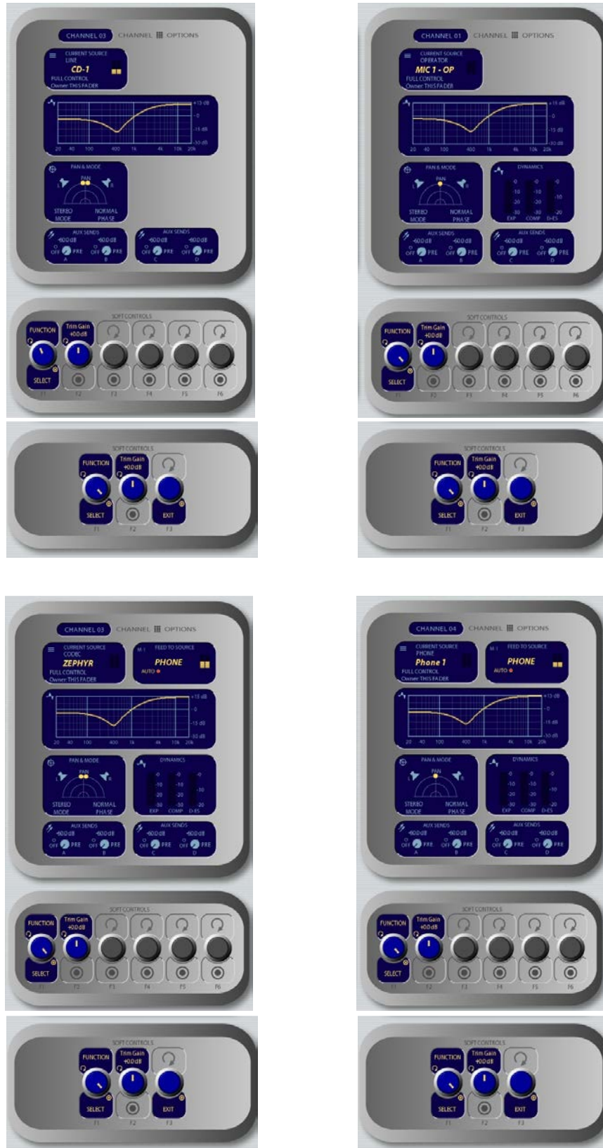
Figure 5-7: Channel Options screens. Information displayed differs based on the type of source currently assigned to the active fader. Shown clockwise from top left: Line Source Channel Options screen, Mic Source Channel Options screen, Phone Source Channel Options screen, Codec Source Channel Options screen. 2-Fader controls are shown below.
